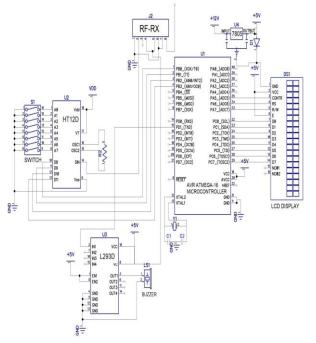
Fig.3 Receiver Section
