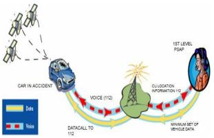
Fig. 12 Alert Data transmission
