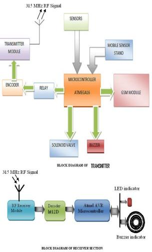
Fig. 1 Block Diagram of Proposed System
